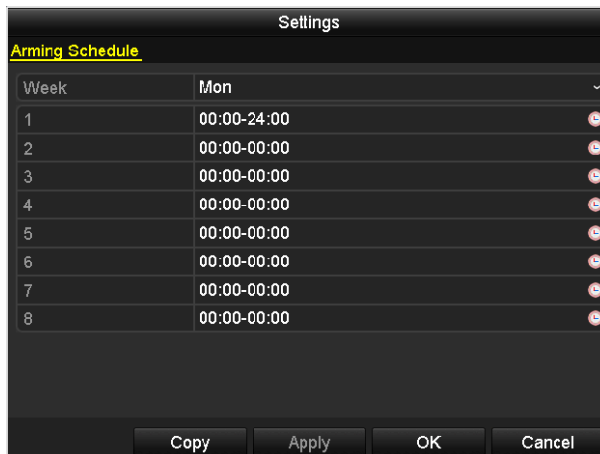
Figure 8-17 Set Arming Schedule of Alarm Output
