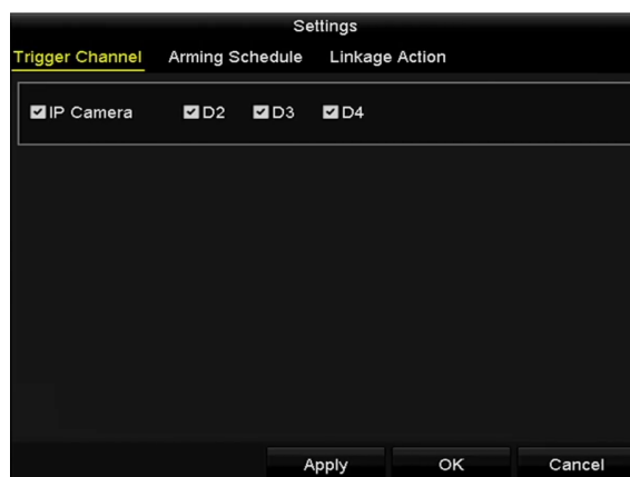
Figure 5-19 Set Trigger Camera of VCA Alarm
